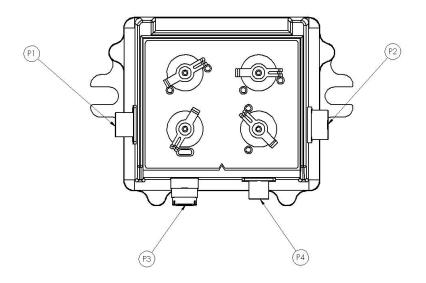
Figure 2.1: FFCS External Connectors
